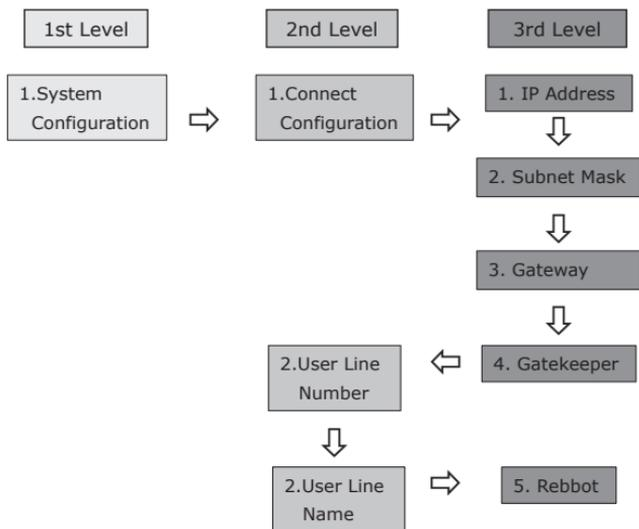
Machine default running mode is P2P mode. If you'd like to connect others via GK mode, the setup procedure of VIP-100T can be referred below:
