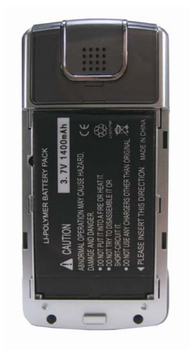
Figure 5. Mounted the battery view
