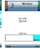
Figure 4-24: Enter WEP Key (for Secured Network)
