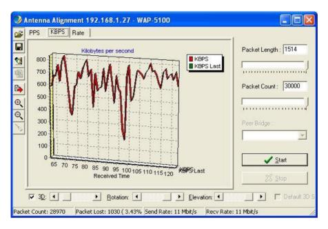
During the antenna alignment test, the bridge might receive interference owing to some unexpected reason. Under this circumstance, the wireless communication data rate will automatically fall back. The numbers of packets sent or received at different data rates can be viewed as shown below.
