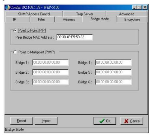
• Point to Multipoint: This is for connecting more than two remote sites. At least one of the WAP-5100 must be set to Point-to-Multipoint mode in such network topology. Other WAP-5100 can be set to either Point-to-Point or Point-to-Multipoint mode. In this mode, up to six other bridges can be connected. Their MAC addresses must be entered here.
