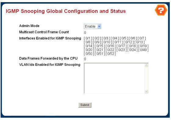
Figure 4-3-19 IGMP Snooping Configuration and Status
