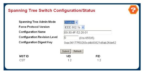
Figure 4-3-33 Spanning Tree Switch Configuration/Status
