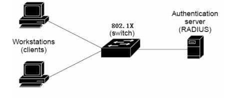
Radius Server — In this situation, need a Radius server in the network, the normal topologies as below
