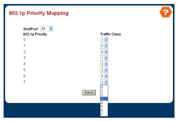
Figure 4-3-40 802.1p Priority Mapping
