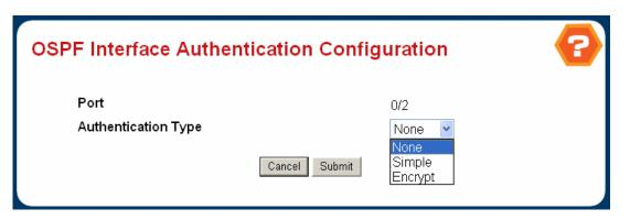
Figure 4-6-18 OSPF Interfac Authentication Configuration
