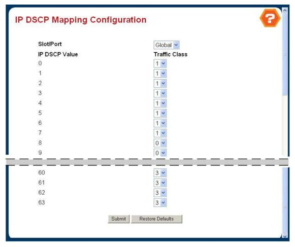
Figure 4-5-28 IP DSCP Mapping Configuation
