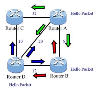
Dead Interval - Enter the OSPF dead interval for the specified interface in seconds. This specifies how long a router will wait to see a neighbor router's Hello packets before declaring that the router is down. This parameter must be
