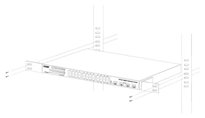
Figure 2-6 Mounting the Switch in a Rack
