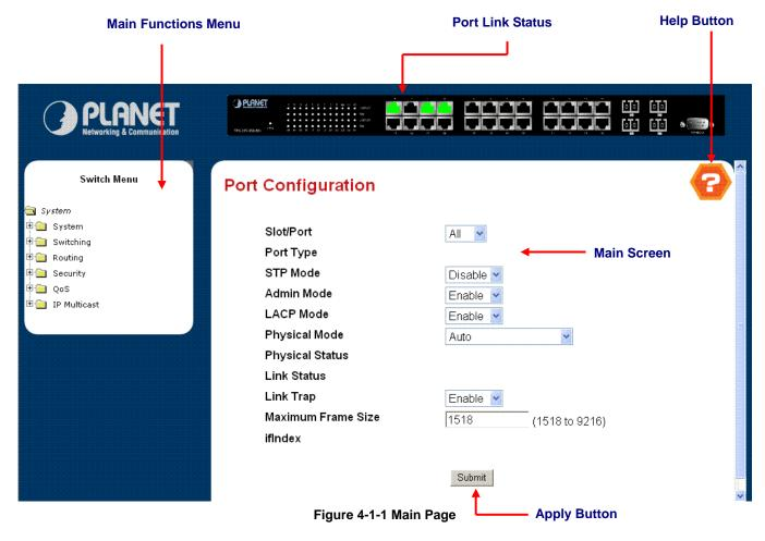
Via the Web-Management, the administrator can setup the WGS3-24000 by select the functions those listed in the Main Function. The screen in Figure 4-2 appears.
