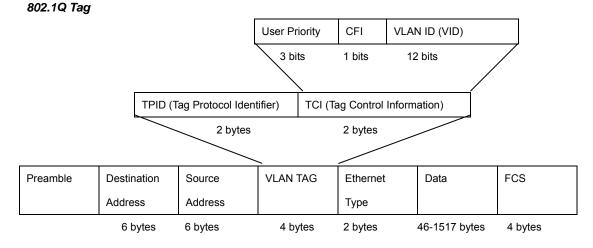
The Ether Type and VLAN ID are inserted after the MAC source address, but before the original Ether Type/Length or Logical
