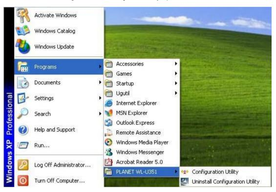
*F.* The Configuration Utility icon will be shown on system tray, if not, that mean the installation is fail. Please uninstall the driver from the system then repeat the installation process.
