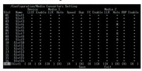
This screen is to set the Device function of LLCF and Link Enable; the Media 1 LLR function, Auto-Negotiation, Speed, Duplex Mode, Flow Control and Link Enable; the Media 2 LLR function, Auto-Negotiation, Duplex mode and Link Enable.
