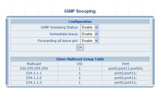
The maximum number of IGMP multicast groups are restricting to 4 entries; the more IGMP Join packets will be filtered.
