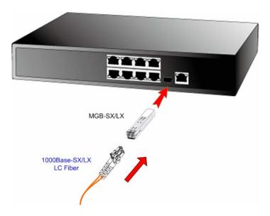
Figure 2-8 Plug-in the SFP transceiver
