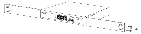
Figure 2-6 Attach brackets to the Switch.
