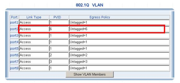
6. Cooperate with IGMP Snooping, and 802.1Q VLAN, Port-6 of VLAN 2 and Port-7 of VLAN 3 are able to receive the Multicast group traffic from Port-2 with different VLAN groups setting
