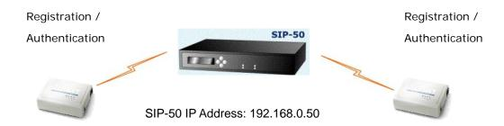
■ ATA A IP Address: 192.168.0.1 ■ ATA B IP Address: 192.168.0.2
