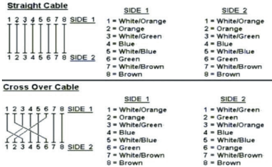
Figure A-1: Straight-Through and Crossover Cable
