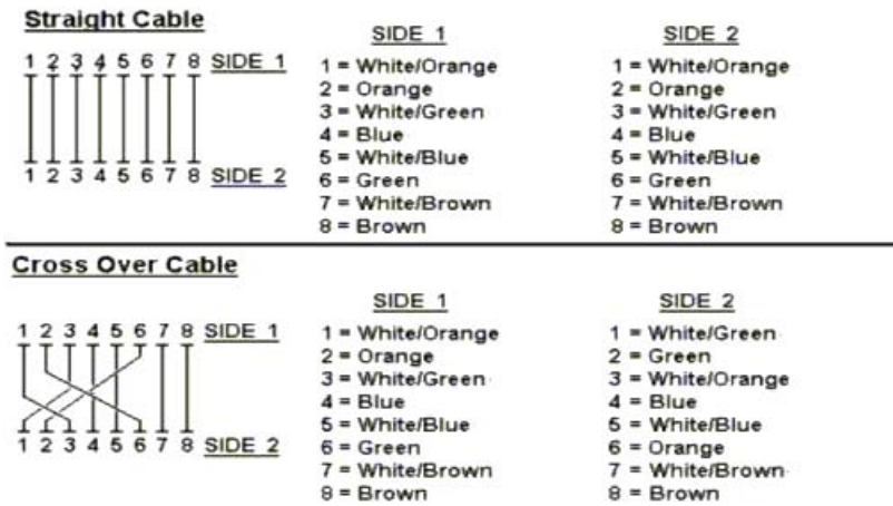
Figure A-1: Straight-Through and Crossover Cable
