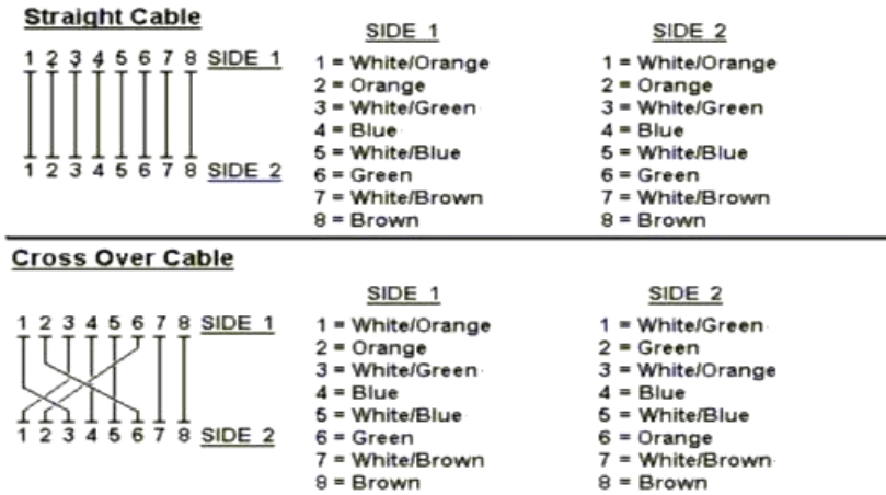
Figure A-1: Straight-Through and Crossover Cable
