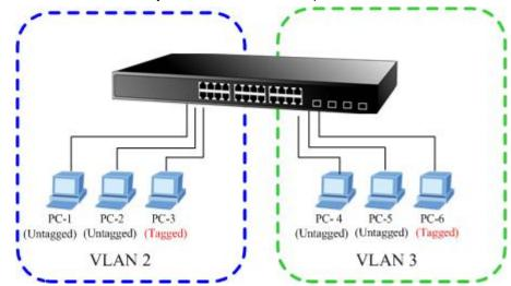
Figure 4-30 two separate 802.1Q VLAN diagram
