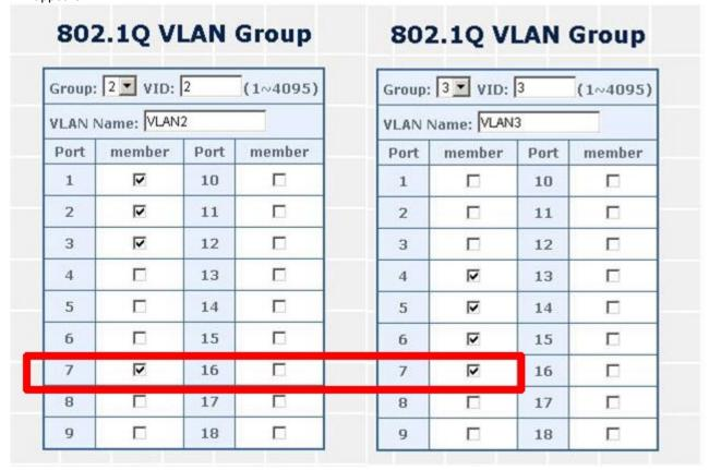
Figure 4-36 VLAN overlap port setting
