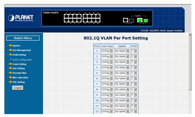
Figure 4-29 802.1Q VLAN per Port Setting Web Page Screen
