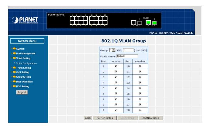
Figure 4-28 802.1Q VLAN Configuration Web Page Screen
