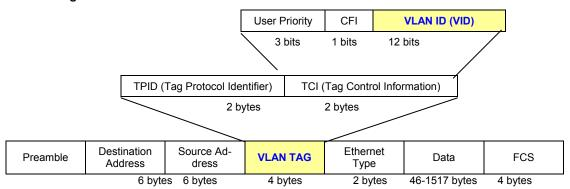
The Ether Type and VLAN ID are inserted after the MAC source address, but before the original Ether Type/Length or Logical Link Control. Because the packet is now a bit longer than it was originally, the Cyclic Redundancy Check (CRC) must be recalculated.
