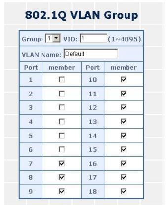
Figure 4-33 Remove specify ports from VLAN 1 member
