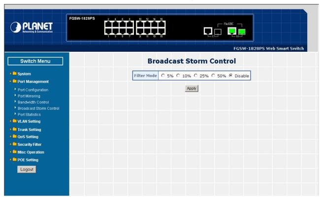
Figure 4-24 Broadcast Storm Control Web Page Screen
