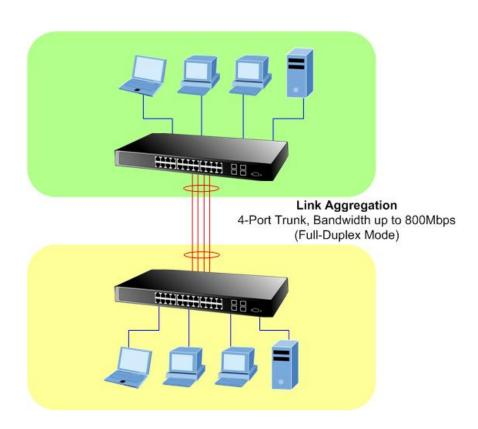
This function allows to configuring the trunk function. It provides up to two trunk groups and each trunk group provides 4 member ports. Also provide four various Trunk Hash Algorithm policies for selection. The screen in Figure 4-42 appears and table 4-16 description the Trunk Setting objects of Web Smart PoE Switch.
