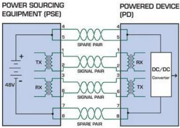
Figure 1 - Power Supplied over the Spare Pins
