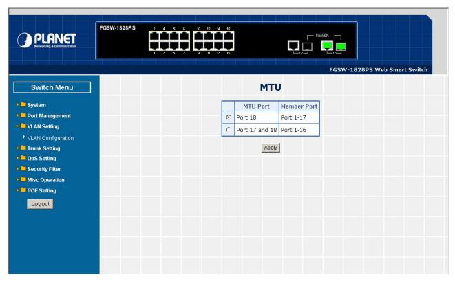
Figure 4-41 MTU VLAN Configuration Web Page Screen
