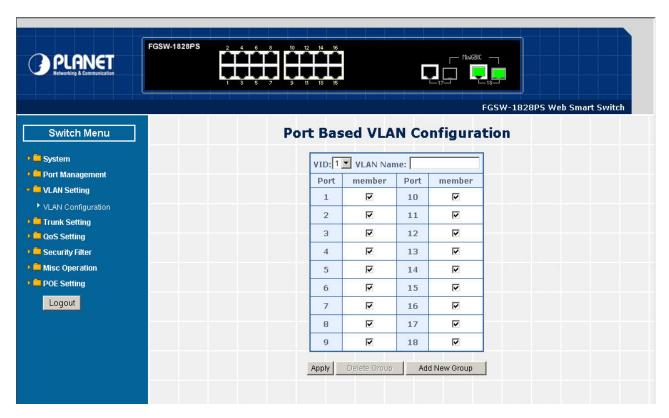
Figure 4-40 Port Based VLAN Configuration Web Page Screen
