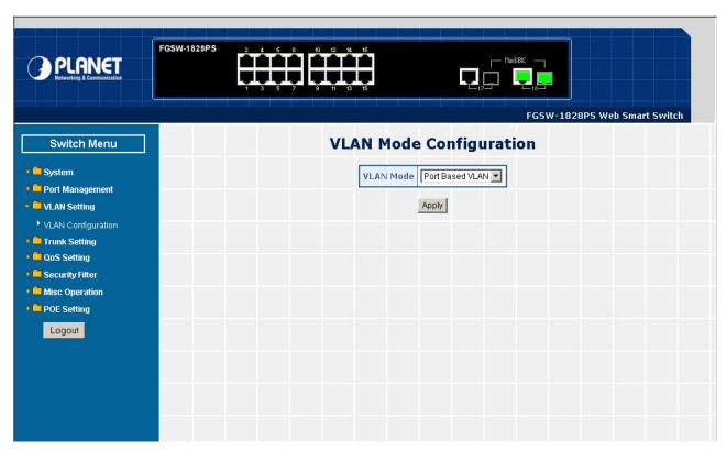
Figure 4-39 Port Based VLAN Configuration Web Page Screen
