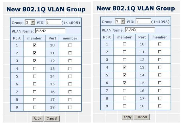
Figure 4-32 Assign VLAN members for VLAN 2 and VLAN 3
