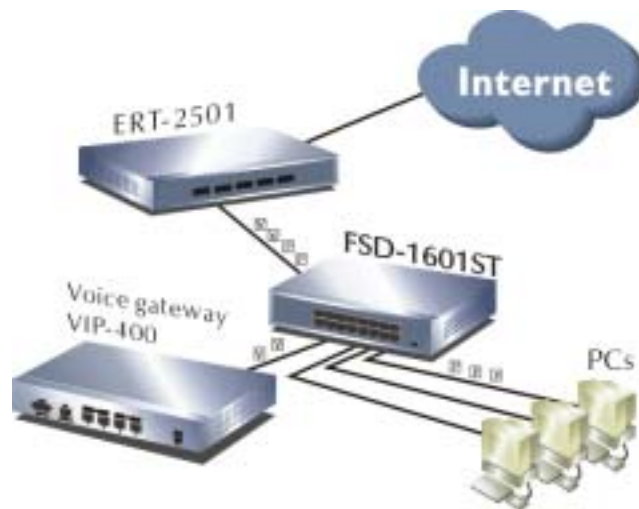
Figure 6. 3 Voice Gateway to Switch Connection
