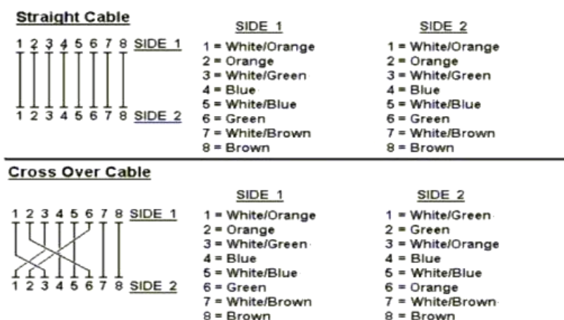
Figure A-1: Straight-Through and Crossover Cable
