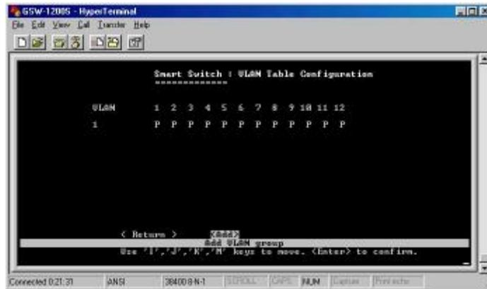
Figure 3-11 VLAN Table Configuration Menu
