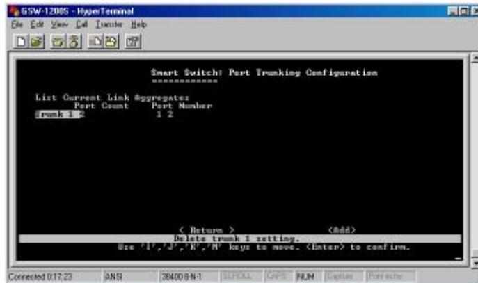
**Figure 3-9** Example of the Defined Trunking Ports
