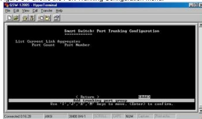
**Figure 3-7** Port Trunking Configuration Menu
