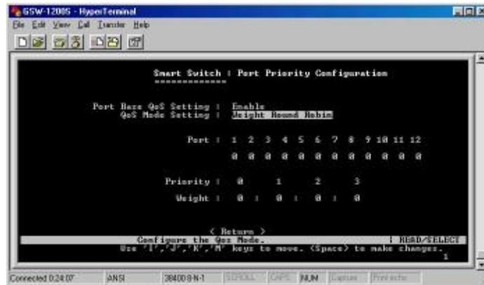
**Figure 3-15** Port Priority Weight Round Robin Configuration Menu Screen
