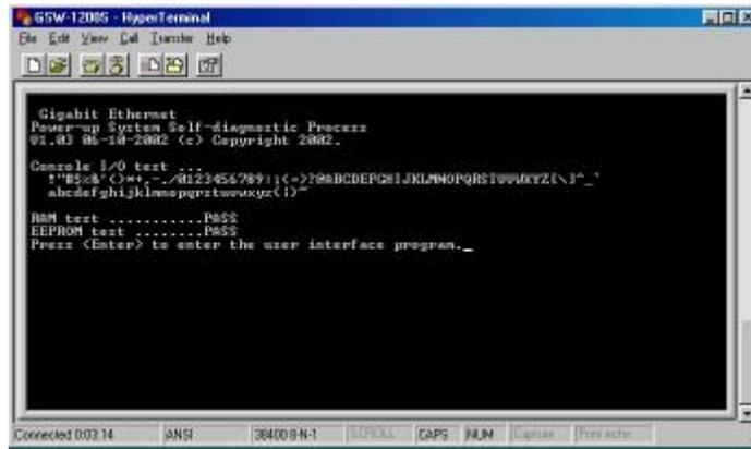
Figure 3-2 Self-test menu of the Power-up System Self-diagnostic Process
