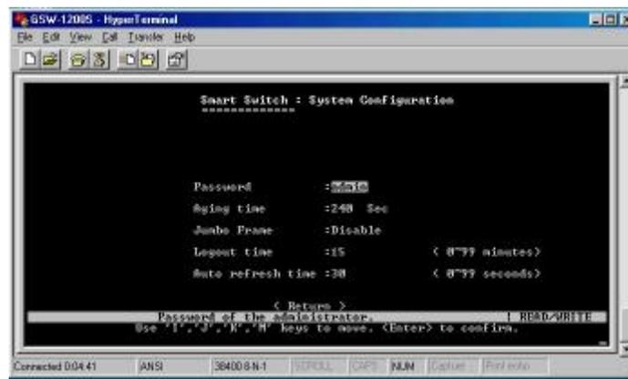
Figure 3-5 System Configuration Menu Screen
