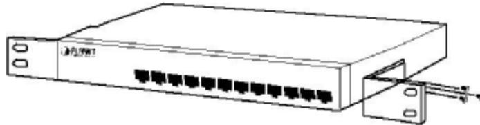
**Figure 2-3** Attaching the brackets to the GSW-1200S
