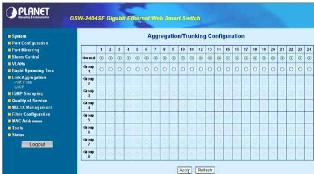
Figure 4-29 Aggregation/Trunking Configuration screen
