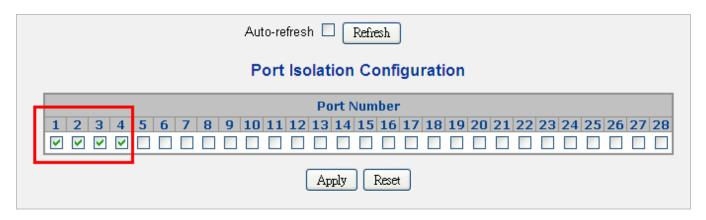
Figure 4-6-17: The Configuration of Isolated and Promiscuous Port
