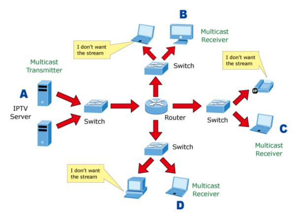
Figure 4-8-2: Multicast Flooding
