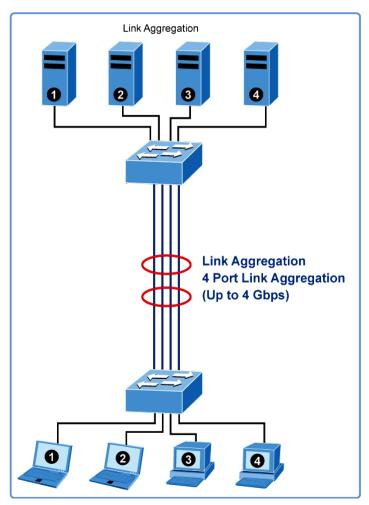
Figure 4-5-1: Link Aggregation Topology
