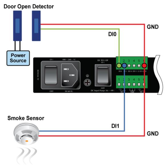
Figure 2-1-11 Wires DI0 and DI1 to Open Detector
