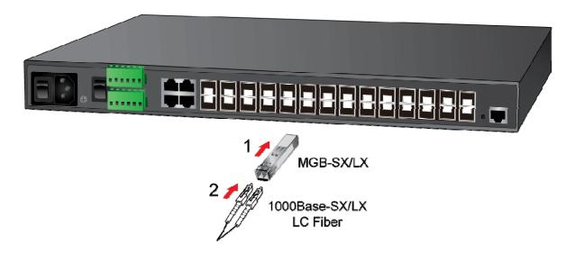
Figure 2-3-1: Plugging in the SFP Transceiver
