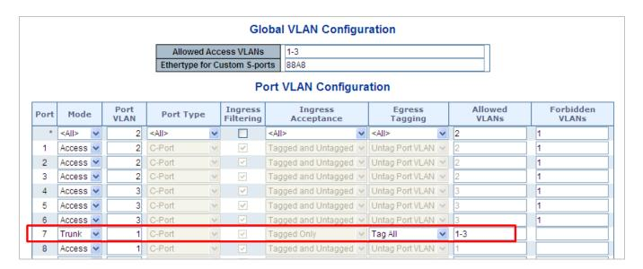
Figure 4-6-15: VLAN Overlap Port Setting & VLAN 1 – The Public Area Member Assign
