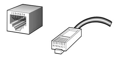
The standard RJ45 receptacle/connector
