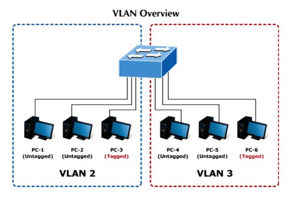
Figure 4-6-8: Two Separate VLAN Diagrams
