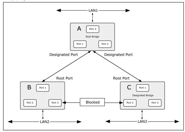
Figure 4-7-3: After Applying the STA Rules
