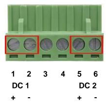
Figure 2-1-8 6-Pin Terminal Block Power Wiring Input
