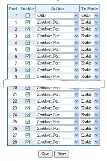
Figure 4-16-1: Loop Protection Configuration Page Screenshot
