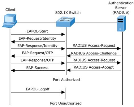
Figure 4-11-2: EAP Message Exchange
