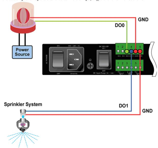
Figure 2-1-12 Wires DO0 and DO1 to Open Detector
