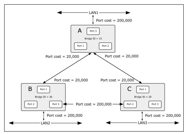
Figure 4-7-2: Before Applying the STA Rules
