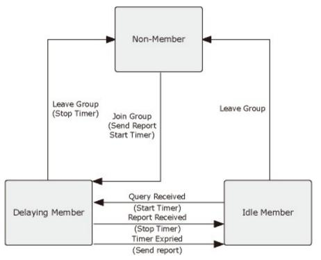
Figure 4-8-4: IGMP State Transitions
