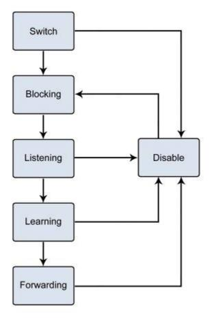
Figure 4-7-1: STP Port State Transitions
