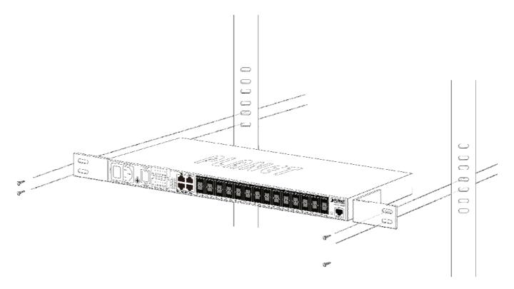
Figure 2-2-3 Mounting the Managed Switch on a Rack
