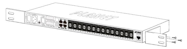
Figure 2-2-2 Attaching Brackets to the Managed Switch.
