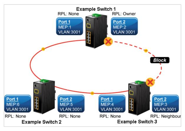
Figure 4-19-6: Ring Example Diagram
