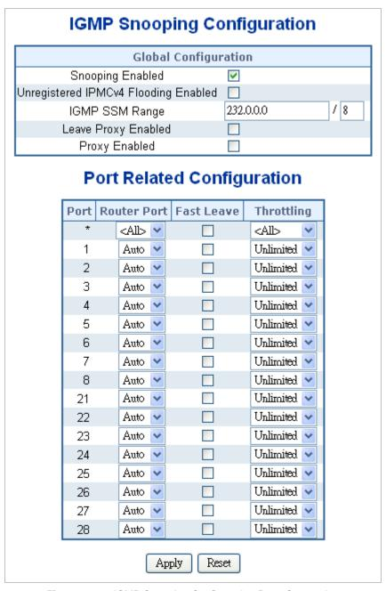
Figure 4-8-7: IGMP Snooping Configuration Page Screenshot
