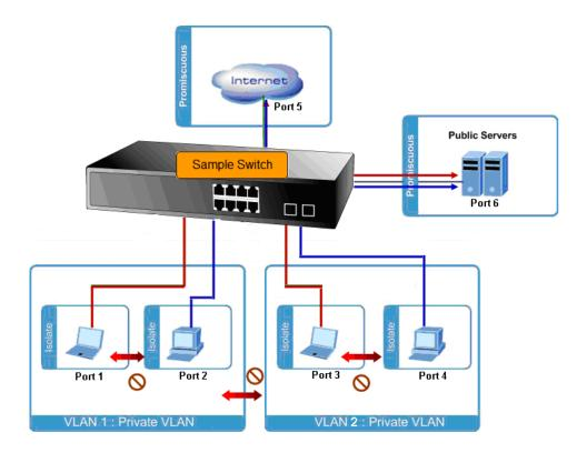
Figure 4-6-16: The Port Isolate VLAN Diagram
