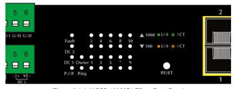
Figure 2-1-4: MGSD-10080F LED on Front Panel
