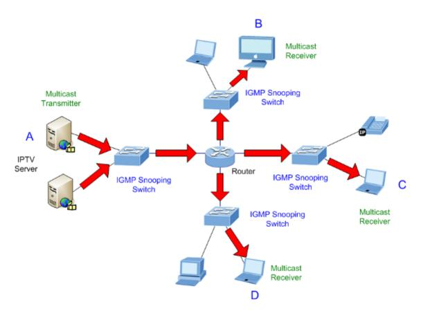
Figure 4-8-3: IGMP Snooping Multicast Stream Control
