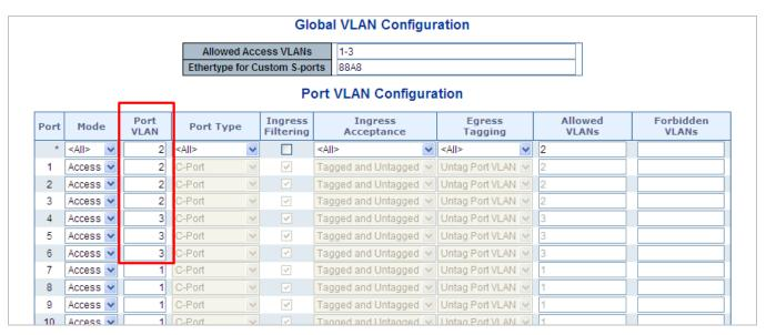
Figure 4-6-10: Change Port VLAN of Port 1~3 to be VLAN2 and Port VLAN of Port 4~6 to be VLAN3
