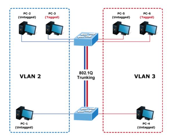
Figure 4-6-12: VLAN Trunking Diagram
