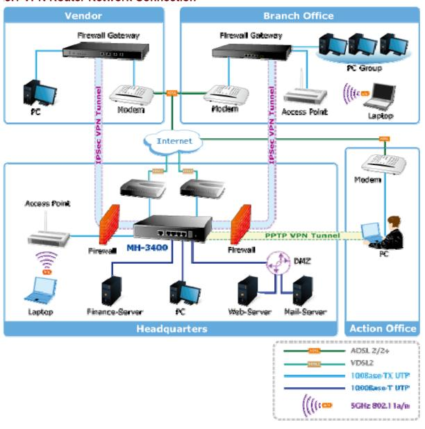
**WAN Connection**: A WAN port can be connected with xDSL Modem, Fiber Modem, Switching Hub, or through an external router to connect to the Internet.
