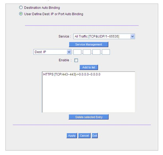
When any intranet IP connects with TCP443 port or any destination (0.0.0.0 to 0 represents any destination), it will go through the same WAN IP. As for which WAN will be selected, this follows the first- chosen WAN IP distributed by the original session balance mechanism.
