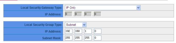
This Local Security Gateway Type must be identical with that of the remote type (Remote Security Gateway Type).
