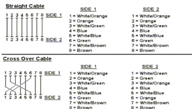
Figure A-1: Straight-Through and Crossover Cable
