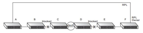
When non-ERPS device protection is enabled on the ring, the ring ports on the RPL
