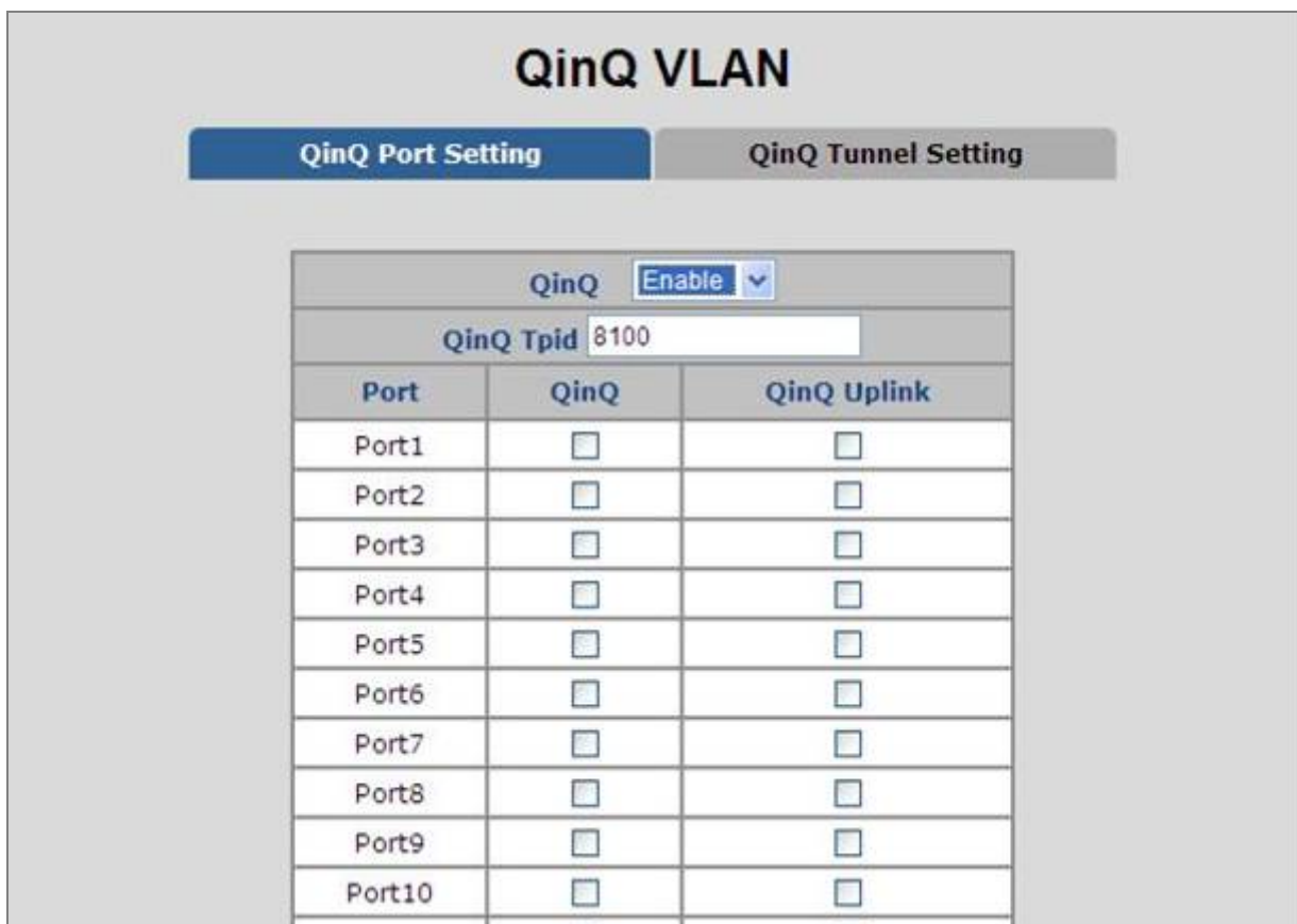
Figure 4-4-8: Q-in-Q Port Setting interface
