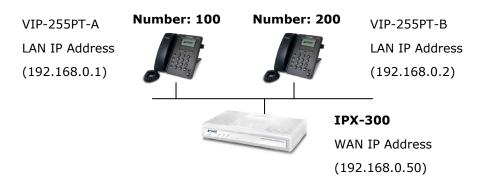
Figure 26.. Installation example with IPX-300
