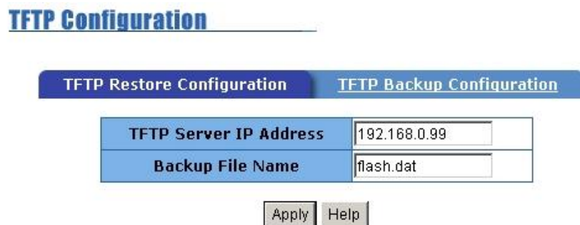
Figure 5-47 WGSD-1020 TFTP Restore Configuration Web Page screen
