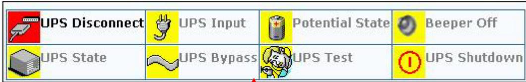
The figure represents the UPS status, when the status has been detected, the figure color change from yellow to red and the status description will be changed.
