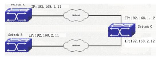
The configuration of Switch C is as follows: (Switch A and Switch B may have the different command because of different companies, we not explain there, our switches are not support NTP server at present)
