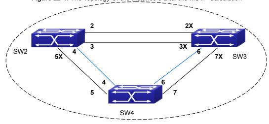
Figure 22-5: The Topology Of the Instance 4 after the MSTP Calculation
