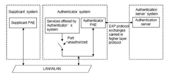
Figure 42-1: The Authentication Structure of 802.1x
