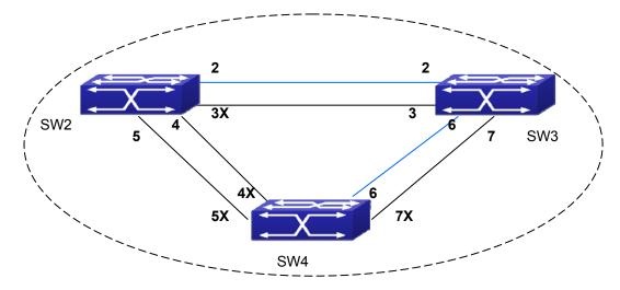
Figure 22-4: The Topology Of the Instance 3 after the MSTP Calculation
