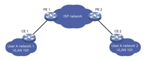
Figure 18-2: BPDU Tunnel application environment
