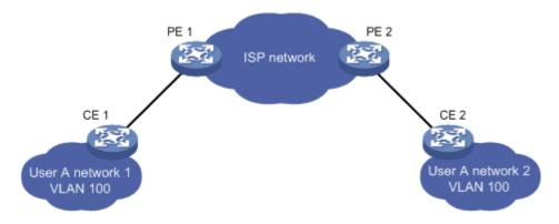
Figure 18-1: BPDU Tunnel application
