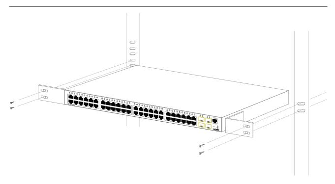
Figure 2-6 Mounting WGSW-52040 in a Rack
