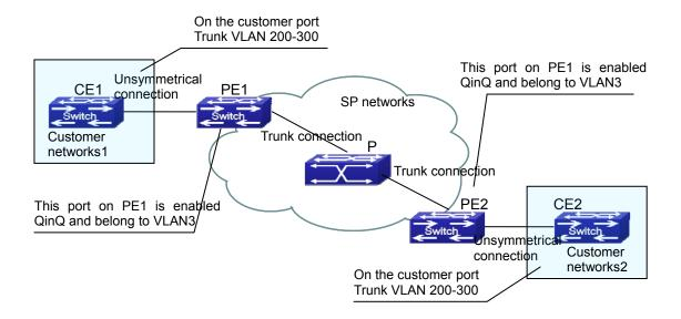
Figure 20-4: Dot1q-tunnel based Internetworking mode
