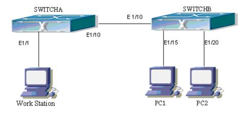
Figure 40-1: Function configuration of the Multicast VLAN
