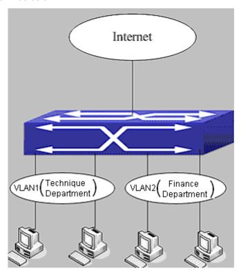
Figure 53-1: VLAN-ACL configuration example
