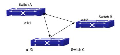
Figure 10-2: One End of Each Fiber Not Connected
