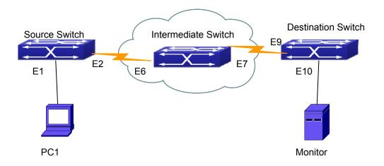
Figure 60-1: RSPAN Application Sample
