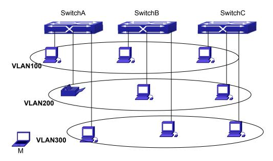
Figure 20-8: Typical topology application of dynamic VLAN
