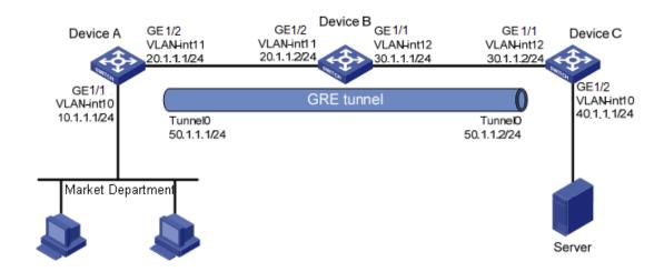
Figure 61-1: ERSPAN application diagram
