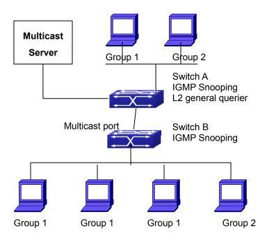
Figure 38-2: The switches as IGMP Queries
