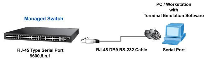
Figure 3-1 Out-of-band Management Configuration Environment
