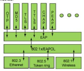
Figure 42-8: the Protocol Stack of EAP Authentication Method
