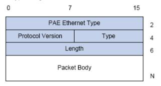
Figure 42-3: the Format of EAPOL Data Packet
