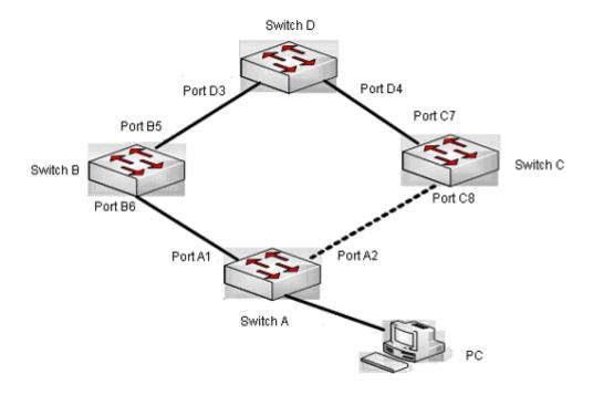
Figure 56-1: the using scene of ULPP
