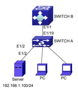
Figure 27-1: ARP scanning prevention typical configuration example
