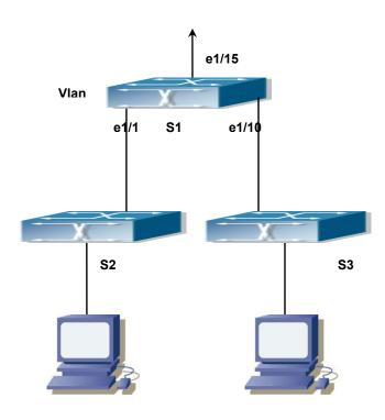
Figure 8-1: Typical example of port isolation function
