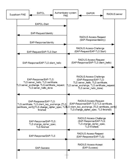
Figure 42-10: the Authentication Flow of 802.1x EAP-TLS
