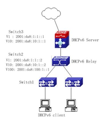
Figure 35-2: DHCPv6 relay option schematic
