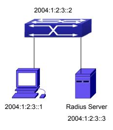
Figure 47-3: The Topology of IPv6 Radius configuration
