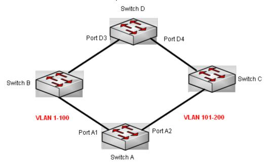
Figure 56-2: VLAN load balance
