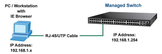
Figure 3-6 Manage the switch by Telnet
