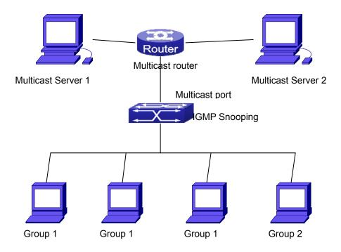
Figure 38-1: Enabling IGMP Snooping function
