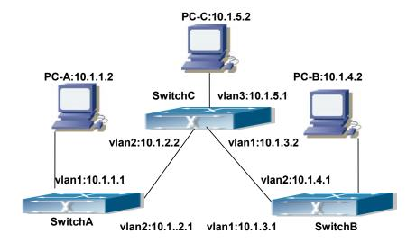
Figure 26-1: Static Route Configurations
