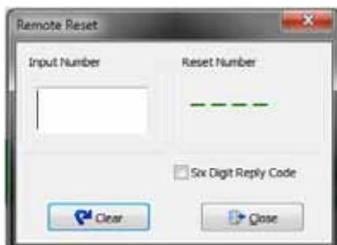
Enter the number that you require to decode in the Input Number box. The Remote Reset number is then displayed in Reset Number Box.
