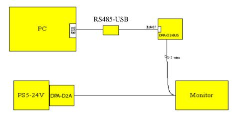
2. Power the system. Now on the PC, Run the DT-Analyzer software. When first run the DT-analyzer, please go to setting and select the port number for USB-485 converter. Here it is COM2.
