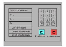
• Maximum 3 telephone numbers can be set, touch the telephone number frame, then input the the number by touching the digital keypad.
