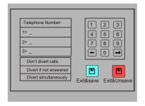
• Maximum 3 telephone numbers can be set, touch the telephone number frame, then input the the number by touching the digital keypad.
