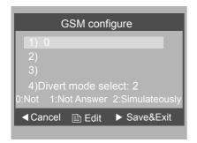
• Maximum 3 telephone numbers can be set,Use ▲ /▼ Button to move upward / downward to select the item,then press the MENU button to edit.Use ▲ /▼ Button to increase / decrease the value,and use ▶ button to input next digital,use ▶ button to ◀ button to cancel the input. press the MENU button again to finish the edit operation.
