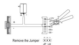
set to Normally Closed on the Unlock Relay mode on DT-config software.
