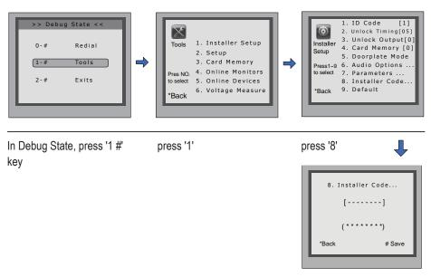
Input a new Installer Code and then press '#' key to confirm
