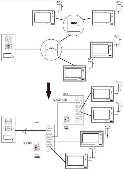
Note1:SET-3Y set to 75R when the distance from door station to the first BDU is within 50 meters, otherwise set to 150R.
