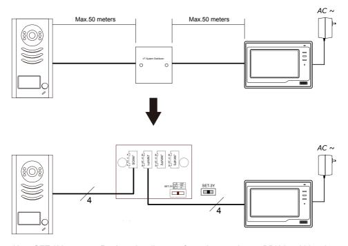
Note:SET-3Y set to 75R when the distance from door station to BDU is within 50 meters,otherwise set to 150R.
