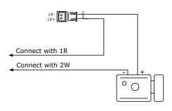
The lock can be directly connected with the door station and the power through monitor. During unlock operation, the monitor will close screen automatically.
