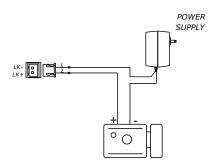
Must install external power supply for lock,and nearly all kinds of electronic lock can be used. Incidentally,in this mode,you can continue talking and monitoring during unlock operation.
