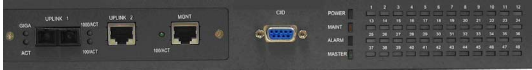
Figure 1-5 ADSL2/2+ IP DSLAM LED Identification
