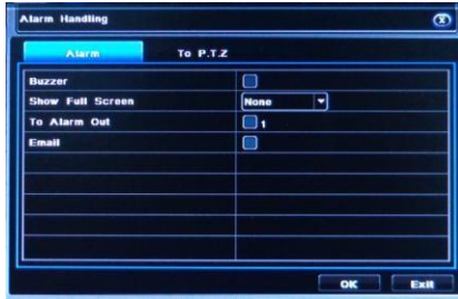
Pic 2-25 Video loss - alarm handling
