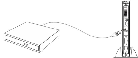
Step2. Put your operating system disk in the external USB device.
