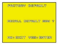
Press 《MENU/OK》 button, returns all settings to the factory default value (NOTE 1). Press 《ESC/STOP》 button, exit this screen display and returns to the Main Menu.
