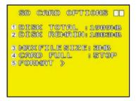
TOTAL SPACE : SD card total capacity. REMAIN SPACE : SD card remaining capacity.
