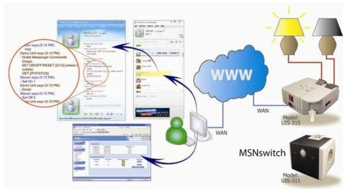
Fig.3 MSNswitch (UIS-311, UIS-315 & UIS-323x) setup for remote control via MSN messenger or thru Web User Interface.
