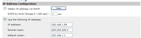
**Obtain IP address via DHCP**: This allows the IPM-401H to automatically obtain a IP Address from the server. *Recommended for non-advance users*.
