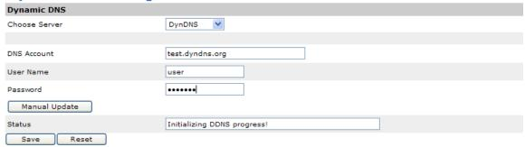
The DDNS section allows you to setup the IPM-401H with a DDNS server (i.e. <a href="https://www.dyndns.com">www.dyndns.com</a>). After the server has been setup correctly, enter the necessary information into the IPM-401H DDNS settings.
