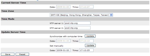
The Date and time section, is where you can set the time and date of the IPM-401H. There are four sections:
