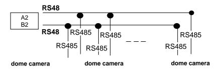
▲ When dome camera is furthest away from the control keyboard, Please set switch of matching resistance as ON status. <sup>3.</sup> R is on behalf of matching resistance. The farthest dome from the control center should be set as its matching resistance in order to minimize RS485 bus reflection and disturbance. The 8<sup>th</sup>bit of SW3 shows ON status which means the BUS matching resistance has been connected.
