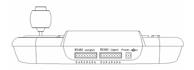
Power supply outlet: connecting external DC9V power.
