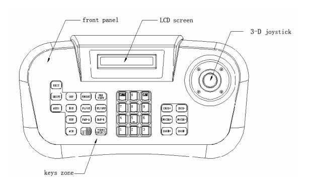
On the front panel of the DVR keyboard are 3-D variable-speed controlling joystick, keys and LED digital displayer. The LED digital displayer shows system and operation information. The controlling joystick controls the different direction variable-velocity movement of the dome as well as the focus length of the lens.
