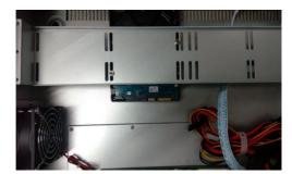
(3) Connect the power & data cable to the NVR and HDD.
