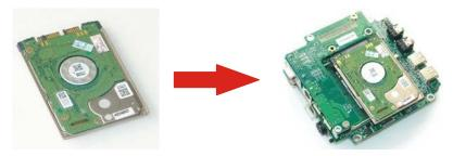
5: Install the finished expansion board into chassis and fix HDD with the drive bays.
