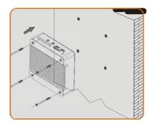
2: The following diagram shows machine of screw holes will be installed hehind the display.
