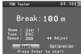
Built-in BNC, network cable, RVV control cable, Telephone line can test. 12 groups user-defined cable can be set.
