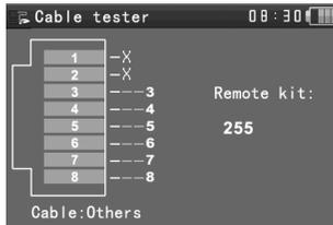
Test LAN cable or telephone cable.
