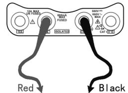
c. Connect test leads in series with the load under measurement.
