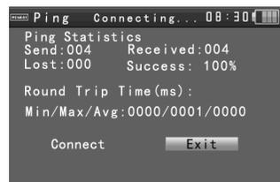
equipment's ethernet port is working normally and the IP address is correct.
