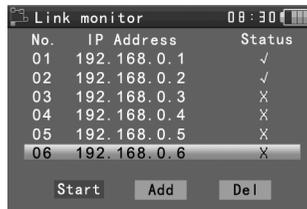
Add the IP address, make sure the network segment and the setting IP address are consistent, choose “start”, and press
