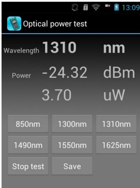
There are six wavelengths as calibration wavelength, choose corresponding wavelength can test current optical
