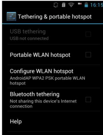
Click "Configure WLAN hotspot" to configure the SSID, security mode and password of the WIFI hot, as follows:
