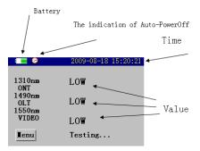
There are the measurement results of three wavelength appearing on the screen, i.e.: 1310nm upstream test and 1490nm/1550nm downstream test. The measurement value will appear when there is light passing through the optical channel, otherwise "LOW" will appear.
