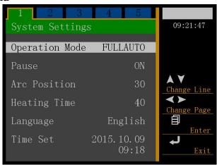
Press the keys " $\blacktriangle$ ", " $\blacktriangledown$ " to move the cursor; press the key to enter the program that you want to get into; press again the keys " $\blacktriangle$ ""  $\blacktriangledown$ " to modify the parameter values (via moving the cursor in the small pane); and press the key to confirm, so that the modification has completed.
