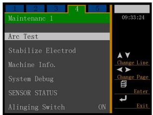
Press "▲" "▼" to move the cursor, press to enter the program that you desire to get into, press "▲" "▼" over again to modify the parameter values(via moving the cursor in the small pane); and press the key confirm, so that the modification has completed. Then, press to quit.
