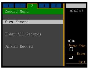
Press to enter "View Record" Menu, and press "\( \delta \)", "\( \bullet \)" to select and view the Fusion-Splicing Records. Under this menu, it is possible to view the Fusion-Splicing Records for operating 6000-times.
