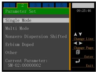
Press "▲" "▼" to move the cursor, and press to enter the "Fusion Splicing Mode" program that you want to get into.
