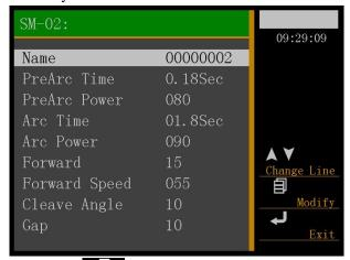
Press "▲" "▼" to move the cursor; press to enter the menu which needs to be modified; press "▲" "▼" to modify the parameters; Press over again to confirm and save it. After completing the modification, press to exit.
