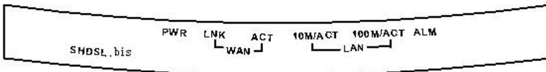
Front Panel of SHDSL .bis 1-port router/bridge
