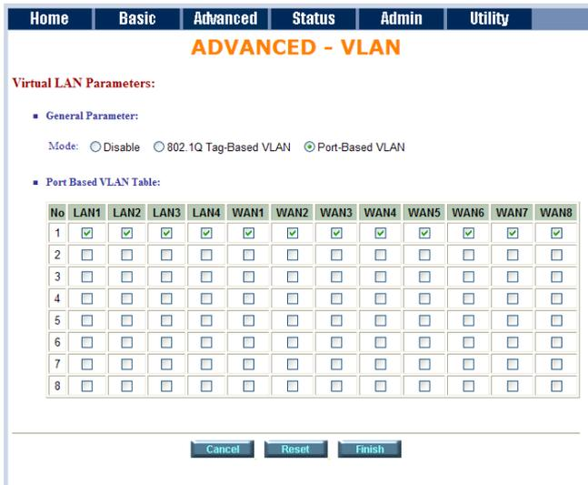
Port-Based VLANs are VLANs where the packet forwarding decision is based on the destination MAC address and its associated port.
