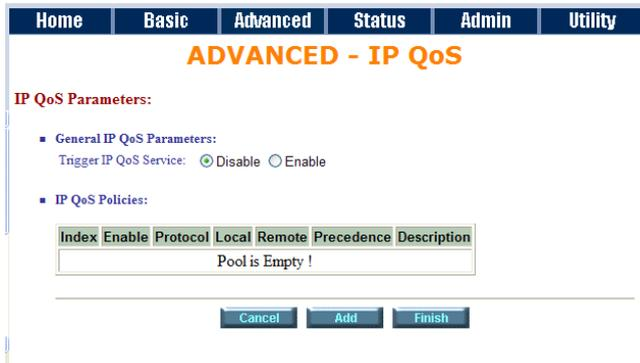
Click **Enable** at item **Trigger IP QoS Service** in General IP QoS Parameter, which will turn on this IP QoS function.
