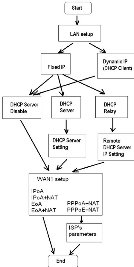
Routing mode contains DHCP server, DHCP client, DHCP relay, Point-to-Point Protocol over ATM and Ethernet and IP over ATM and Ethernet over ATM. You have to clarify which Internet protocol is provided by ISP.
