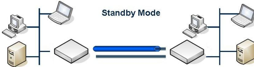
Only one of two pairs are working, other pair is standby. If the working pair fails, the standby pair will start up to continues.
