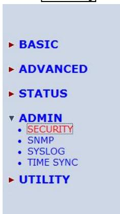
For greater security, change the Supervisor ID and password for the router. If you don't set them, all users on your network can be able to access the router using the default Supervisor IP and Supervisor Password is "**root**".
