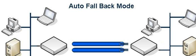
Two DSL pairs are working simultaneously. When one pair of both is disconnect, the other pair will keep working.
