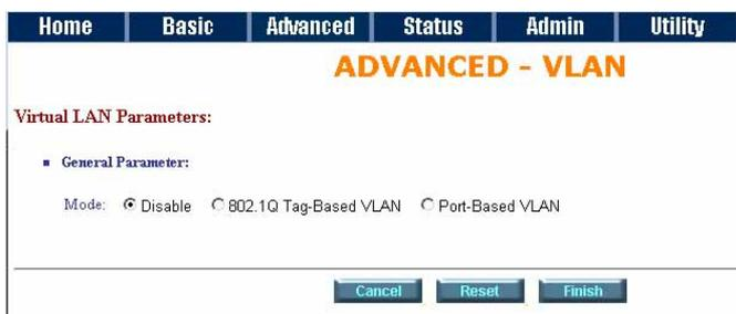
The router supports two types of VLAN: **802.1Q Tag-Based VLAN** and **Port-Based VLAN**. User can configure one of them to the router.
