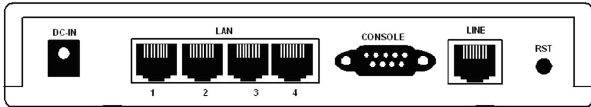
Rear Panel of SHDSL.bis 4-wire/2-wire,4-port router/bridge
