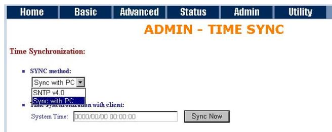
For using the SNTP, select **SNTP v4.0**.
