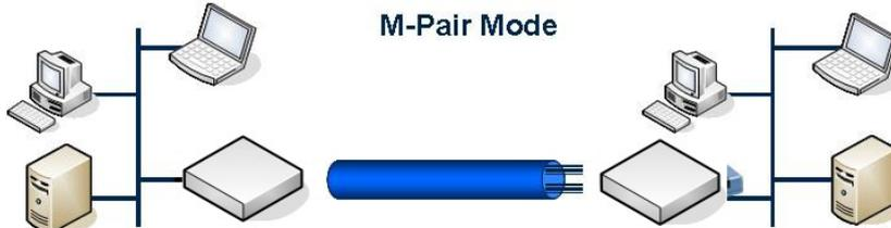
In this mode, each wire pairs of SHDSL.bis router must be configured with the same line rate. If one pair fails then the entire line must be restarted. It also has the Conexant M-pair standard used with connection to other router with Conexant chip set solution.
