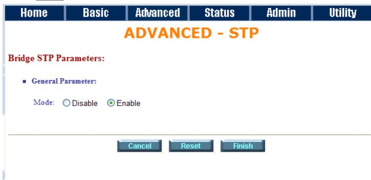
STP (Spanning-Tree Protocol) defined in the IEEE 802.1D, is a link management protocol that provides path redundancy while preventing undesirable loops in the network. For an Ethernet network to function properly, only one active path can exist between two stations.
