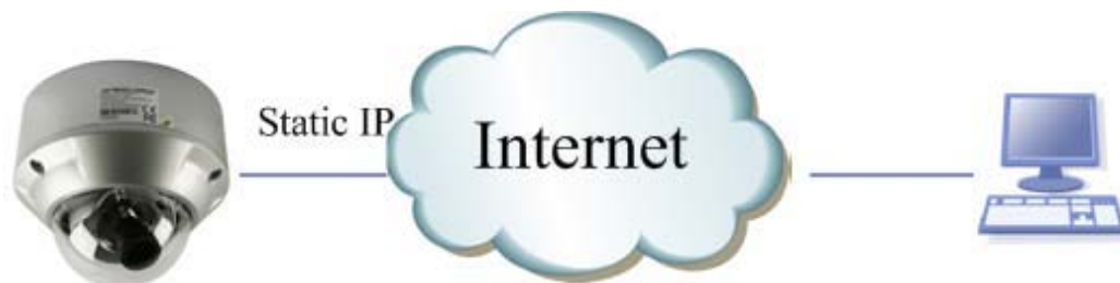
Fig.3.5.2 Static IP access IPC directly
