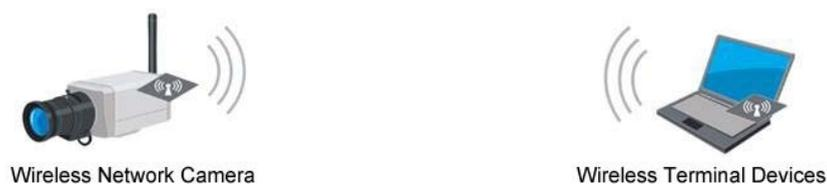
Fig. 1.2.1 Peer-to-peer Communication Through Wireless Network
